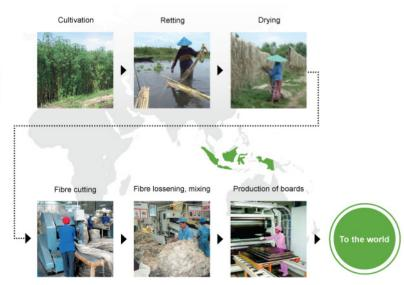
We commercialised a start-to-finish system for kenaf from caltivation to production of pre-board, a base material used in car interiors in Indonesia. We supply kenaf to our factories manufacturing interior components around the world.
